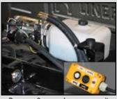
Power up & power down power unit with 10' tethered control box
